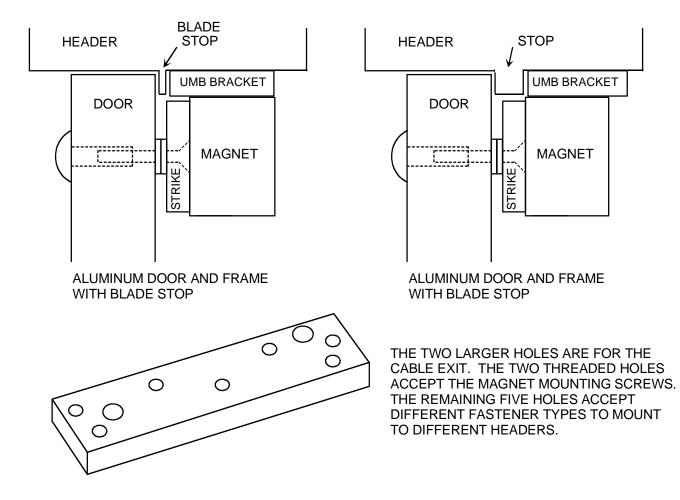
NOTE HOW BRACKET CAN BE REVERSED TO COPE WITH DIFFERENT STOP THICKNESSES
